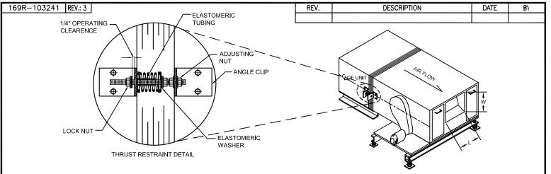
THE THRUST FORCE CREATED BY A FAN IS A FUNCTION OF THE TOTAL STATIC PRESSURE AND THE CROSS SECTIONAL AREA OF THE FAN OUTLET. TO ESTIMATE THRUST FORCE, USE THE FOLLOWING FORMULA:
