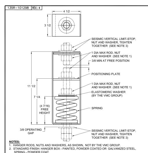
3. SEISMIC VERTICAL LIMIT-STOP REQUIRED FOR SEISMIC APPLICATIONS. NOT BY THE VMC GROUP. INSTALL WASHER .165 THK, MIN. X 2-1/2 O.D. MIN. WITH REQUIRED INSIDE DIAMETER TO ACCOMMODATE ROD SIZE IN USE. THIS CAN BE ACCOMPLISHED BY USING A SINGLE WASHER OR BY STACKING NOT MORE REV. DESCRIPTION DATE BY
