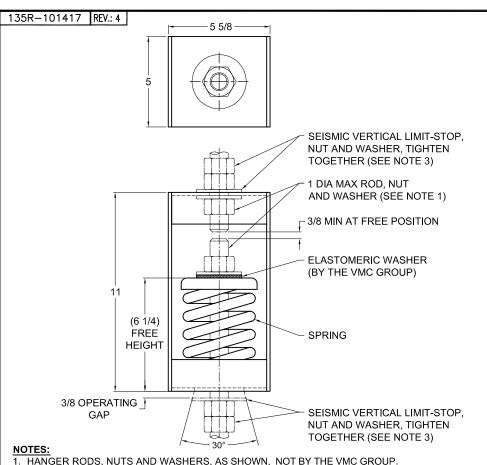
2. STANDARD FINISH: HANGER BOX - PAINTED, POWDER COATED OR GALVANIZED STEEL
