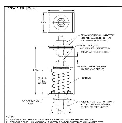
3. SEISMIC VERTICAL LIMIT-STOP REQUIRED FOR SEISMIC APPLICATIONS. NOT BY THE VMC GROUP. INSTALL WASHER .134 THK. MIN. X 1-3/4 O.D. MIN. WITH REQUIRED INSIDE DIAMETER TO ACCOMMODATE ROD SIZE IN USE. THIS CAN BE ACCOMPLISHED BY USING A SINGLE WASHER OR BY STACKING NOT MORE
