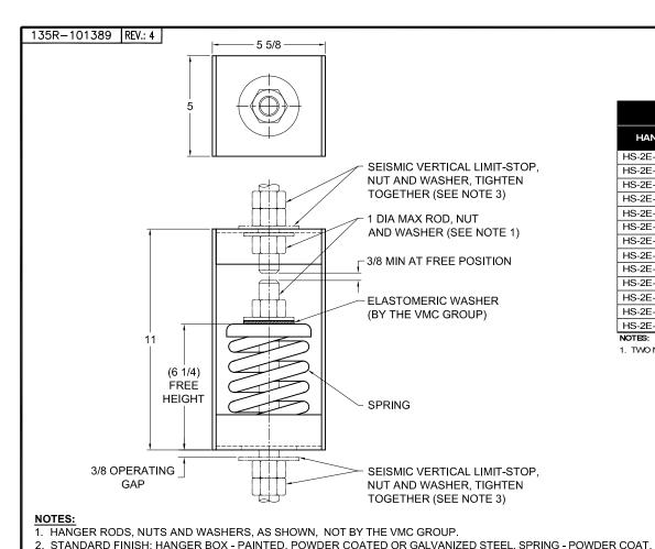
SEISMIC VERTICAL LIMIT-STOP REQUIRED FOR SEISMIC APPLICATIONS. NOT BY THE VMC GROUP. INSTALL WASHER .16 THK. MIN. X 3 O.D. MIN WITH REQUIRED INSIDE DIAMETER TO ACCOMMODATE ROD SIZE IN USE. THIS CAN BE ACCOMPLISHED BY USING A SINGLE WASHER OR BY STACKING NOT MORE
