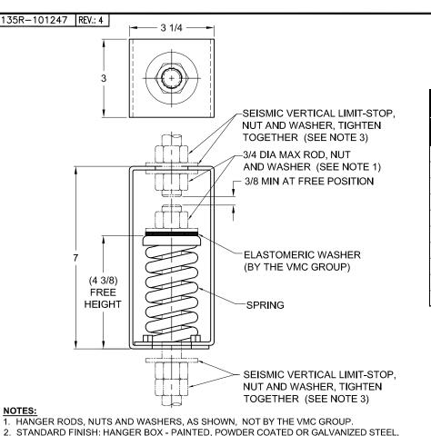
3. SEISMIC VERTICAL LIMIT-STOP REQUIRED FOR SEISMIC APPLICATIONS. NOT BY THE VMC GROUP. INSTALL WASHER .148 THK. MIN. X 2 O.D. MIN WITH REQUIRED INSIDE DIAMETER TO ACCOMMODATE ROD SIZE IN USE. THIS CAN BE ACCOMPLISHED BY USING A SINGLE WASHER OR BY STACKING NOT MORE
