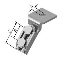
**Installation:** Use SB-125's with standard 1-5/8" strut, ASTM A-307 Grade A bolt, and standard washer when directly attaching to building structure.
