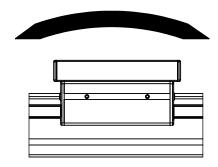
$M_y$  (static) = 131 in-lbs, 15 Nm.  $M_y$  (dynamic) = 209 in-lbs, 23 Nm.
