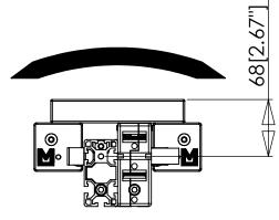
$M_x$  (static) = 182 in-lbs, 20 Nm.  $M_x$  (dynamic) = 292 in-lbs, 33 Nm.
