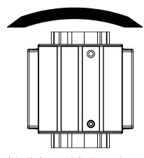
$M_z$  (static) = 442 in-lbs, 50 Nm.  $M_z$  (dynamic) = 708 in-lbs, 80 Nm.
