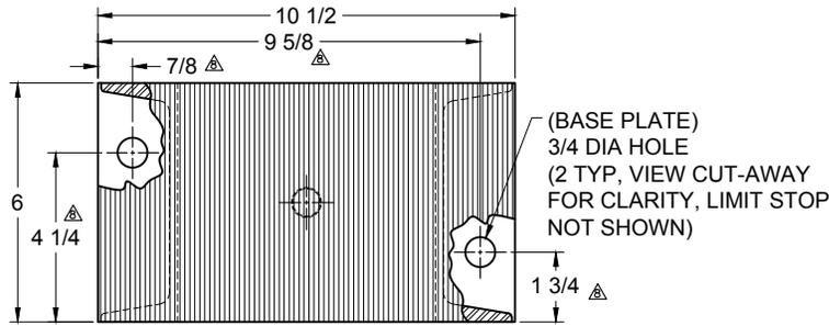
**TYPE MT-3D SPRING ISOLATORS WITH INTERNAL ADJUSTMENT AND ELASTOMERIC PAD-COVERED TOP PLATE**
