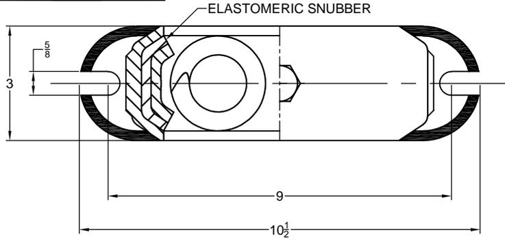
**TYPE C2DE-2B CAST IRON SPRING-FLEX MOUNTINGS WITH EXTERNAL ADJUSTMENT**
