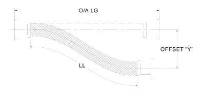
WHERE OFFSET MOTION "Y" OCCURS BOTH SIDES OF THE CENTERLINE, THE HOSE LIVE LENGTH SHOULD BE BASED ON TOTAL TRAVEL OF 2 TIMES "Y".
