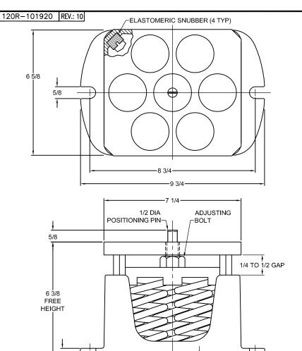
2. FINISH: HOUSINGS- CAST IRON, SPRINGS- POWDER COAT, HARDWARE: ZINC-ELECTROPLATE.
