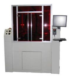
FlexAblaser is capable of fine line and mass ablation of common film polymers. Developed primarily for ITO ablation, this new system is capable of micro-ablating other conductive and non-conductive inks, including silver and carbon. A solid silver, carbon or carbon over silver print can be rapidly converted into a high definition circuit by FlexAblaser. Something impossible to do with conventional screen printing or ink jet processes. Avoid the registration issues with printing carbon over
