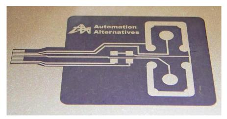
Example of Silver ablation from 5 mil polyester. Excellent for fine line definition of 0.5mm pitch tails and Prototype production.
