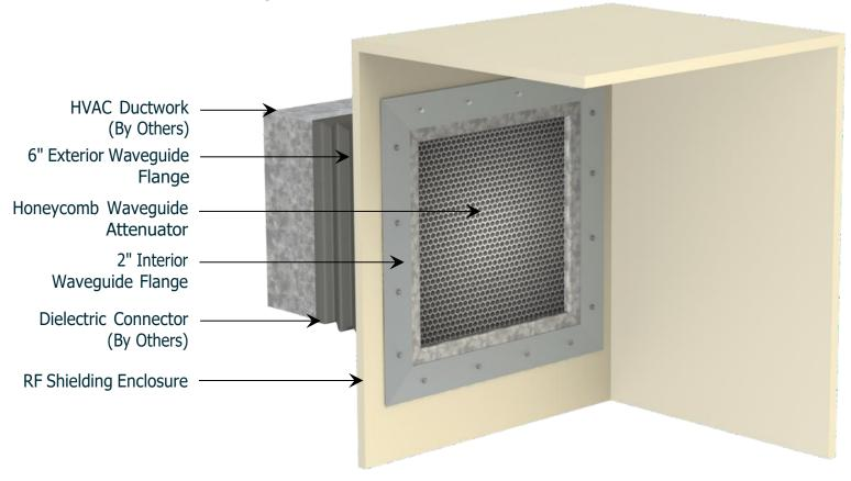
HONEYCOMB CELL [3/16" or 1/8"] x 1" THICK
