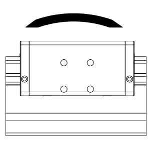
M<sub>y</sub> (static) = 35 in-lbs, 4 Nm. M<sub>y</sub> (dynamic) = 43 in-lbs, 4.8 Nm.
