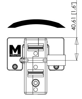
M<sub>x</sub> (static) = 25 in-lbs, 2.8 Nm. M<sub>x</sub> (dynamic) = 32 in-lbs, 3.5 Nm.
