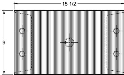
**TYPE MT-5D SPRING ISOLATORS WITH INTERNAL ADJUSTMENT AND ELASTOMERIC PAD-COVERED TOP PLATE**
