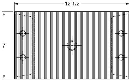
**TYPE MT-4C SPRING ISOLATORS WITH INTERNAL ADJUSTMENT AND ELASTOMERIC PAD-COVERED TOP PLATE**
