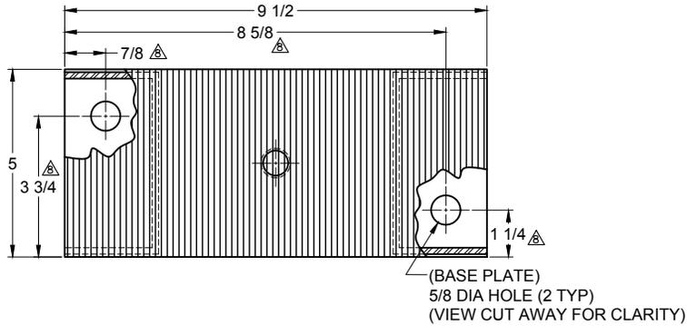
**TYPE MT-3C SPRING ISOLATORS WITH INTERNAL ADJUSTMENT AND ELASTOMERIC PAD-COVERED TOP PLATE**
