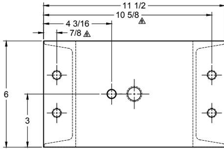
**TYPE MP-3R SPRING ISOLATORS WITH INTERNAL ADJUSTMENT AND POSITIONING PIN**
