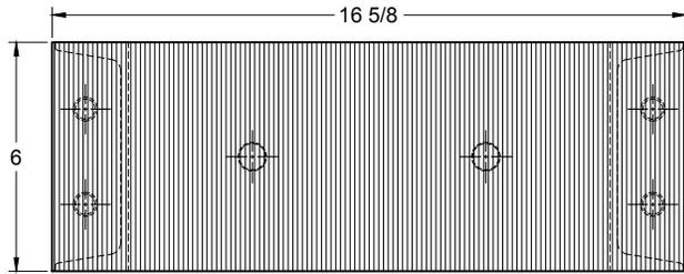
**TYPE M2T-3D SPRING ISOLATORS WITH INTERNAL ADJUSTMENT AND ELASTOMERIC PAD-COVERED TOP PLATE**
