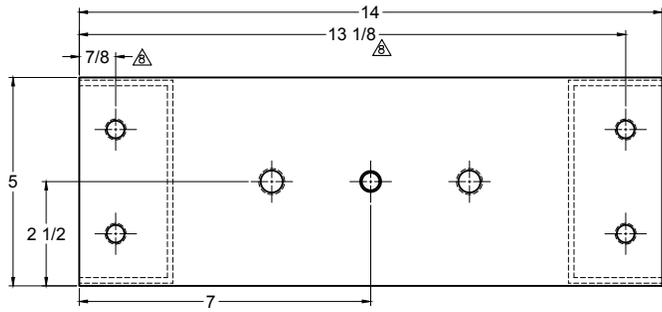
**TYPE M2P-2E SPRING MOUNTS WITH INTERNAL ADJUSTMENT AND POSITIONING PIN**
